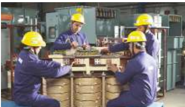
Transformer Fitting Process
